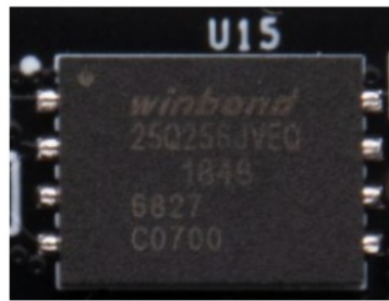
Figure 2-4-2 is the QSPI Flash on the core board
