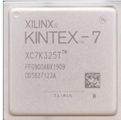
Figure 2-2: FPGA chip on board
