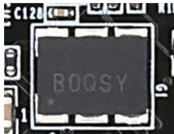
Figure 3-2: 200Mhz Active Differential Crystal on the Core Board
