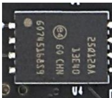
Figure 5-2: QSPI FLASH on the Core Board
