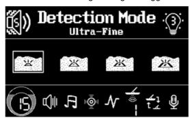
Fine: Fine detection mode reduces sensitivity to mineralised soil and may not detect very small gold nuggets. When paired with the Nugget Finder 12"x7" Mono coil or similar-sized coils, this mode performs exceptionally
