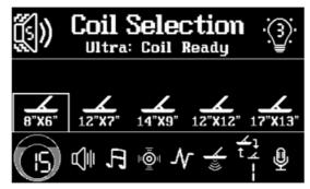
If the package comes with a coil, its calibration parameters will be saved as the default parameters for all the coil icons. If it doesn't, the parameters of a factory-designated standard coil will be used as the default. Factory reset does not change the coil icons' calibration parameters or coil size.
