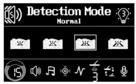
Large: Reserve Large Gold mode for use in extremely mineralised soil with high levels of wet salt. When used with coils larger than the Nugget Finder 14"x9" Mono coil, this mode excels, even in highly mineralised soils. This combination is highly recommended for locating large gold nuggets in different ground conditions.
