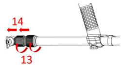
15-16. Align the hole of the coil yoke with the hole of the lower-piece rod. Then attach the coil to the coil yoke and the lower-piece rod.
