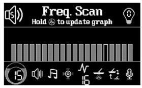
Electromagnetic interference often changes. The past noise levels from the last Auto FS may not accurately reflect the current real-time noise levels. If necessary, hold the Return/Auto FS button to update the past noise level to the current real-time noise level.
