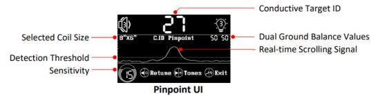
Pinpoint is a non-motion mode where the coil doesn't have to move to indicate a target. The detection signal gets stronger as the coil approaches the target, causing the audio (if audio output is on) or vibration (if vibration mode is on) to intensify.
