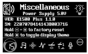
To perform a factory reset, hold both the Minus and Plus buttons for 3 seconds. After a factory reset, the coil profiles, including the coil names and calibration data, remain intact, so you don't need to set up your coils again.
