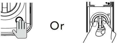
In Manual Mode, the device can be locked by pushing the Multi-Function button on the inside panel or by turning the thumb turn. (Thumb turn will be in the horizontal position when locked)
