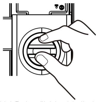
• Turn the thumb turn on inside body (Thumb turn will be in the vertical position when unlocked)
