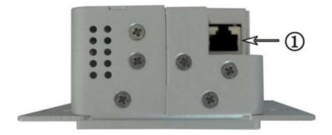
HDBaseT OUT: RJ45 port, connect with receiver via a CAT5e/6 cable to deliver Audio/ Video signals, support PoC.
