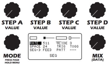
**RATE:** Sets the sequencer step speed, higher numbers are faster.
