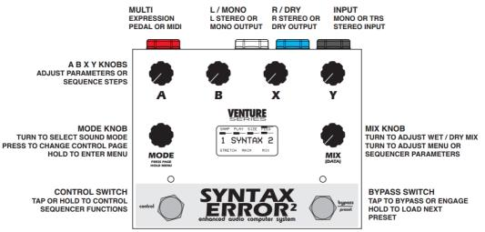
The display shows the current function and position of each knob, as well as the sound mode, preset name, and page name. If you're using an expression pedal, the display will also show the pedal position while it's moving.
