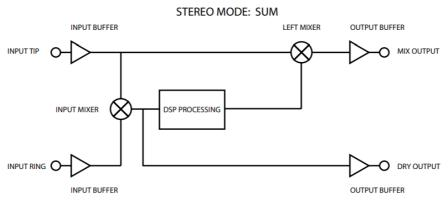
Sum mode combines left and right inputs into a mono signal for processing and outputs a mono signal on the L / MONO output. Useful if you need to sum a stereo source when using a single amplifier.
