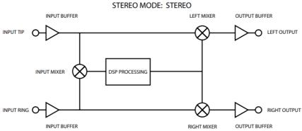
Stereo Mode preserves the separate stereo dry signals. Effect processing is based on the sum of the left and right inputs, and is split to both outputs in most modes. Some modes process the stereo image separately.
