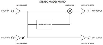
Mono Mode processes the input signal in mono, and outputs a mono signal on the L / MONO output jack. The dry signal is available on the R / DRY output jack.
