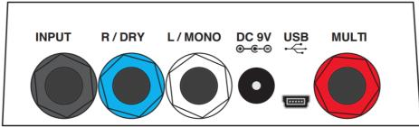
**DC 9V:** Center-negative, 2.1mm ID barrel jack for DC input. The pedal requires a minimum of 250mA to operate, higher current supplies are acceptable. Do not power the pedal from a source greater than 9.6V DC.
