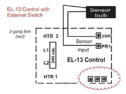
Connect control to external start/stop switch (included) (wire not included). Install the external switch in the one-gang box (not included). Run 18/3 from switch to control. Wire can be 200-300 hundred feet. Do NOT run low voltage wire next to line voltage. The button will switch the sauna on & off. The LED light will come on when the sauna is operating. It will go off when the sauna is off. Will not connect wirelessly via Alexa, Google Home or similar.
