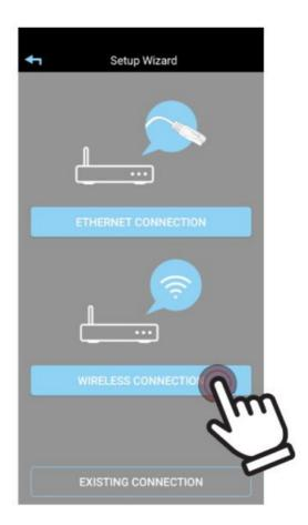
Tap on **Wireless Connection** for WiFi connection. If this camera is already logged on to a device, select **Existing Connection**.
