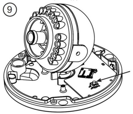
Reset the camera by pressing the reset button for 6 seconds. Indication LED will blink.
