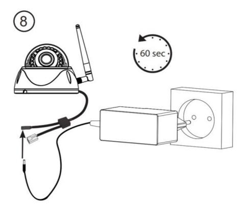
Open the camera and connect the camera to the power supply, and wait at least 60 seconds.
