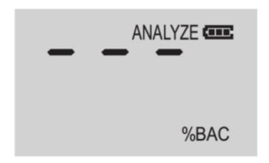
**Step 4.** When the sampling is successful, LCD outer lines will be turning along the edge of the LCD as you can see from the picture.
