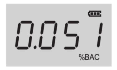
**Step 5.** The estimated BAC (Blood Alcohol Concentration) will flash for 10 seconds, and the button will be deactivated during this time. After waiting for this time, press the power button for 1 second if you want to test again.
