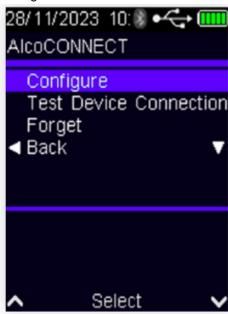
Press the V button, ensure BT is enabled if not already. Press the V button again until page 5 is displayed. The screen will start to populate with devices.
