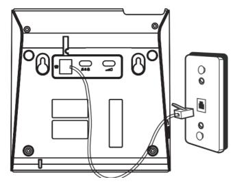
3. Fix the telephone on the wall. (Fig. 5)
