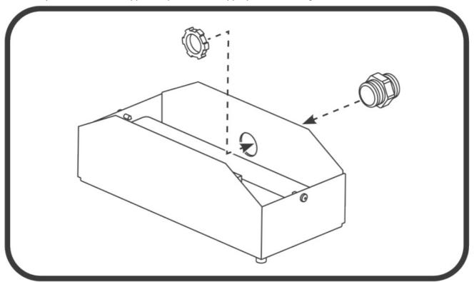
3. Using the attached nipple adapter, mount the EBBM to an appropriate means of mounting (fixture, junction box, conduit, etc.). Ensure that the EBBM is facing downwards
