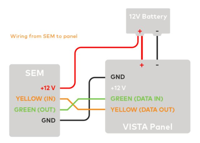
**Important:** If you do not know what this means, disregard this sentence. Alternate wiring is required when using this device for ETL installations. (+12v wire from the SEM will go to the +12V terminal on the panel)
