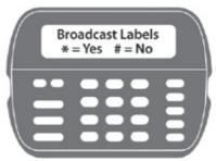
**Broadcast sensor names by selecting the following:** []+[8]+ [Installer Code] + [\*] to enter LCD programming. From LCD programming, go to field 998 and press [] to broadcast sensor names.
