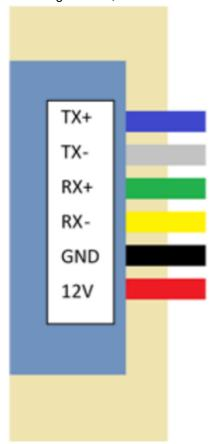
The other end of these wires connect to similarly labeled terminals on the gateway inside the communicator box, but the order of the wires is switched. TX+ and TX- on the communicator remote mounting module should connect to RX+ and RX- on the gateway, respectively. Likewise, RX+ and RX- on the communicator remote mounting
