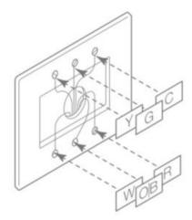
**ACAUTION:** Wiring can vary for each manufacturer. Label all wiring before removing it from the existing thermostat.
