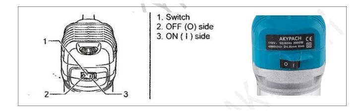
**WARNING!** Never use the tool if its switch cannot turn it on or off smoothly. **WARNING!** Never use tool without the motor installed in the router base.
