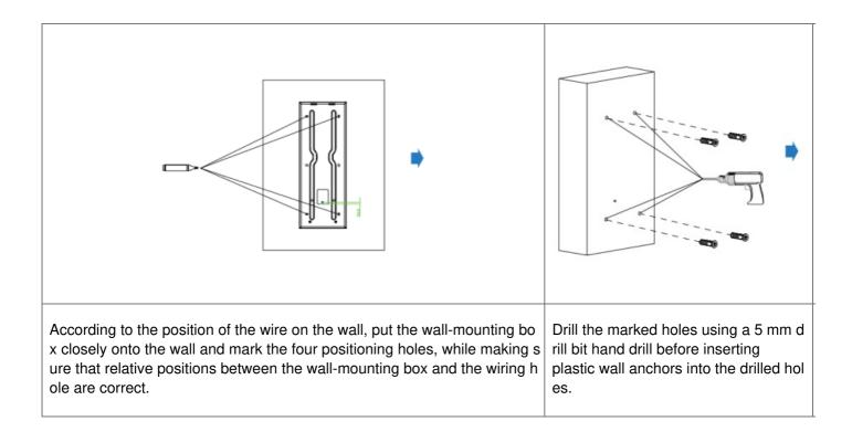
Note: It is suggested that you move the bottom edge of the square hole 10 mm away from the wring hole on the wall as highlighted in green in the drawing.
