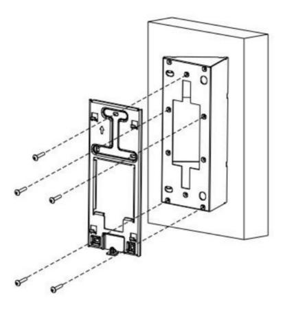
Pace the rotary bracket closely against the wall while lining up its four holes with their corresponding drilled holes. And then fasten the rotary bracket on the wall by tightening four ST4x20 crosshead screws to the plastic wall anchors.
