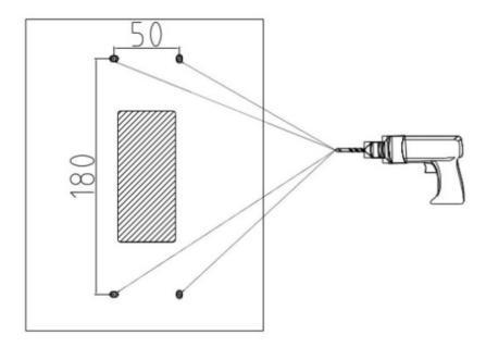
Insert the four plastic wall anchors into the drilled holes.
