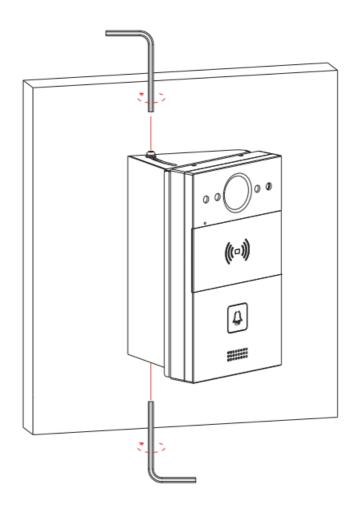
• Fix the M3×8 Torx screws onto the rotary bracket using the Torx wrench, then tighten the screws at the appropriate rotary angle.
