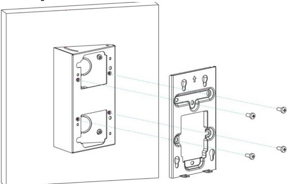
Fix the wall-mounting bracket onto the rotary bracket using four M4×10 screws.
