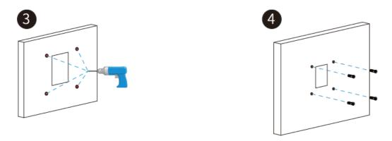
5. Twist M3xI0.5 hex socket screw into the bottom hole of the wall-mounting bracket until the tail of which aligns with the edge. Then fix the wall-mounting bracket on the wall with four ST4x20 crosshead screws. If there is a ground wire to be connected, please use M3x6 crosshead screw to fix it on the wall-mounting bracket.
