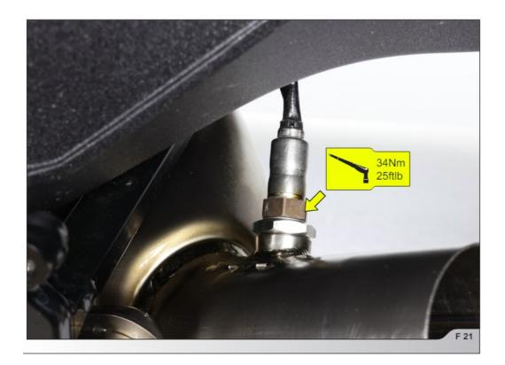
■ IMPORTANT: make sure not to damage the lambda sensors' electrical leads during this process!
