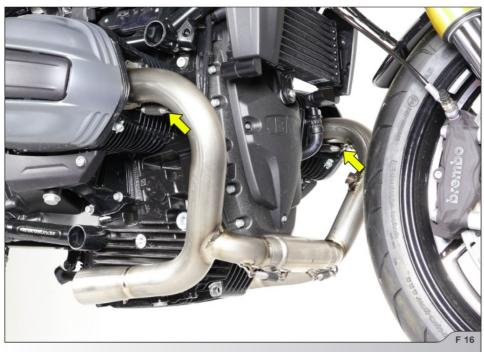
**IMPORTANT:** make sure, that spring pulls the header all the way into the headers sleeves – use rubber mallet if necessary to tap the connections into plac
