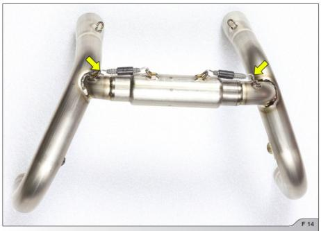
**IMPORTANT:** make sure, that spring pulls the link tube all the way onto the headers – use rubber mallet if necessary to tap the connections into place!
