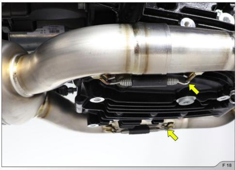
■ IMPORTANT: make sure, that springs pull the pre muffler all the way onto the header tubes – use rubber mallet if necessary to tap the connections into place!
