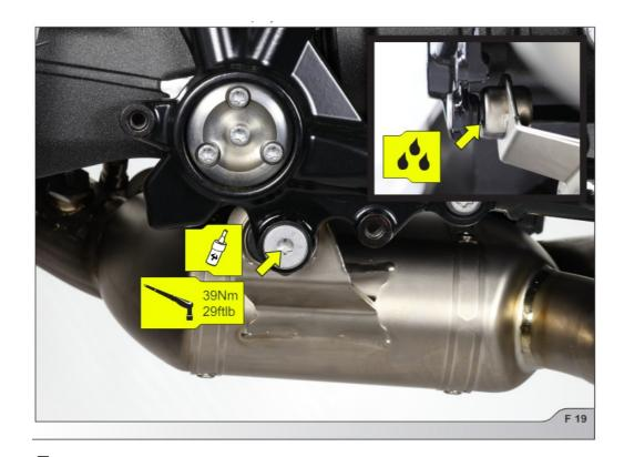
■ IMPORTANT: use bolt sealant on marked bolt threads!
