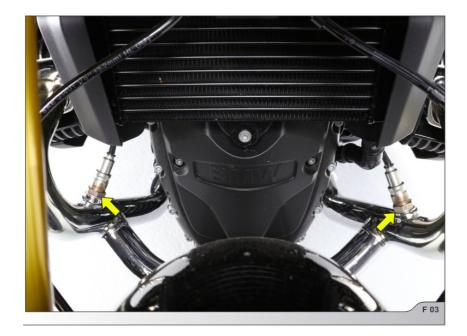
■ IMPORTANT: make sure not to damage the lambda sensors' electrical leads during this process!
