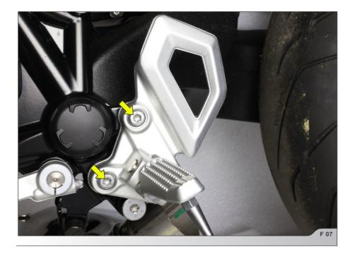
7. Unscrew the marked pre muffler's bracket bolts and remove the header off the motorcycle (F 08, 09).
