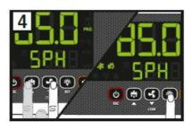
Use keys N and Q to enter the desired moisture Set Point (SPH) value and press SET.
