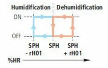
The rH07 parameter allows the dehumidification function to be disabled (rH07 = 0, dehumidification enabled, rH07 = 1 dehumidification disabled). If a dehumidifier has been connected (ln2 = 12, 13 or 14), rH07 is locked at 0; to modify it, choose an ln2 option without a dehumidifier.
