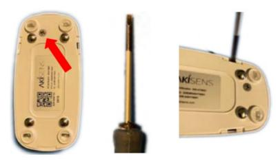
Insert an AA Battery in the sensor and close the cover.
