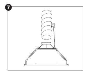
Step 3: Install the insert vent on the hood.
