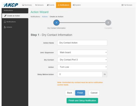
**Note:** The dry contact needs to be connected to the unit before it can be configured, and it needs to be in the Output direction (see below).
