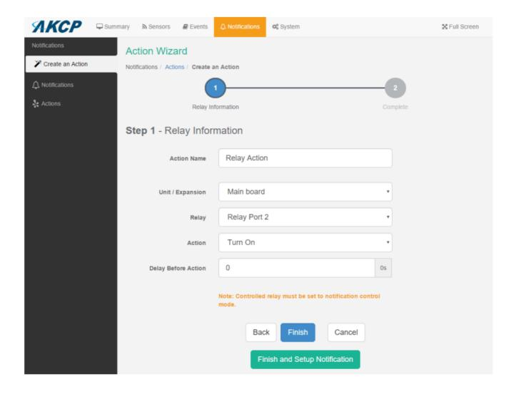
**Note:** The relay needs to be connected to the unit before it can be configured.
