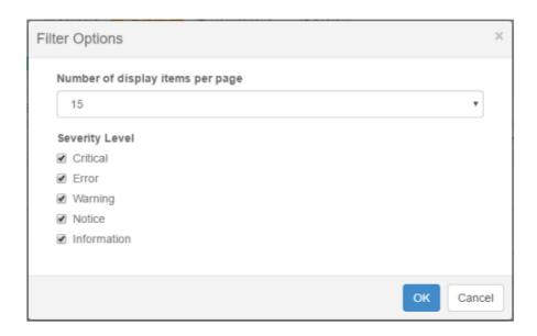
In the Options, you can change the number of log entries displayed per page. The default is 15, it's possible to specify up to 100. Also you can filter by Severity Level.
