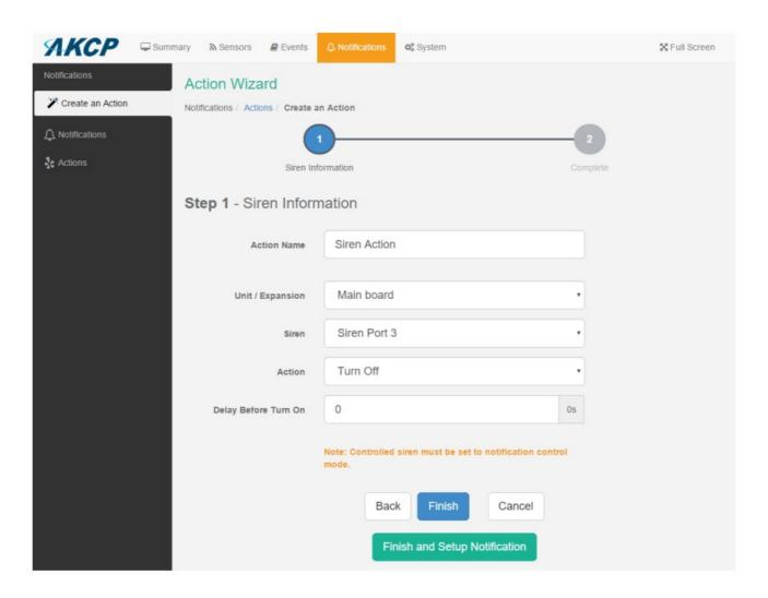
**Note:** The siren needs to be connected to the unit before it can be configured. You'll have the following options for controlling the siren with the action:
