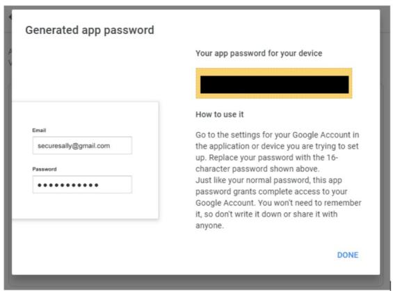
5. The App password is the 16-character code in the yellow bar on your device. Replace your Gmail password on AKCP devices with this password, the other SMTP configurations can be left unchanged. SEC (securityProbe): Edit the Email notification actions in Notification => Action page, edit system SMTP settings in Settings => System Maintenance page. SP+ (SP2+ &SPX+): Edit the SMTP settings in Settings => SMTP page.
