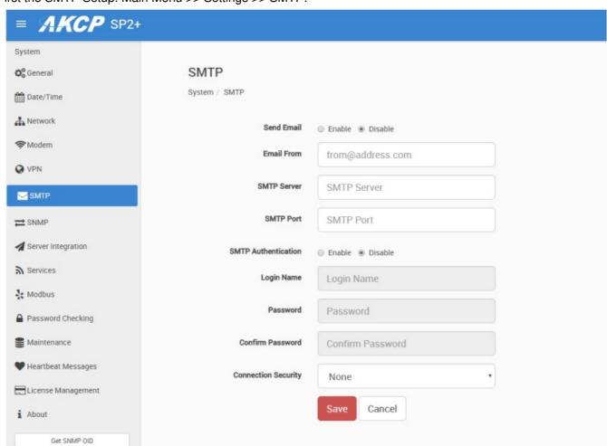
The SMTP server configuration options are shown here, it's required to be set up for the Email actions.
