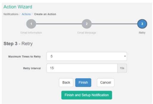
These parameters set the maximum number of times to send the email notification and the time interval between each notification.
