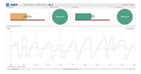
The NIST2 sensors feature 2x NIST traceable, calibrated temperature sensors and an internal calibration integrity check.
