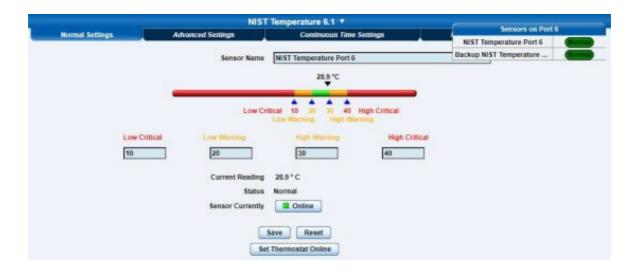
The NIST2 sensors feature 2x NIST traceable, calibrated temperature sensors.
