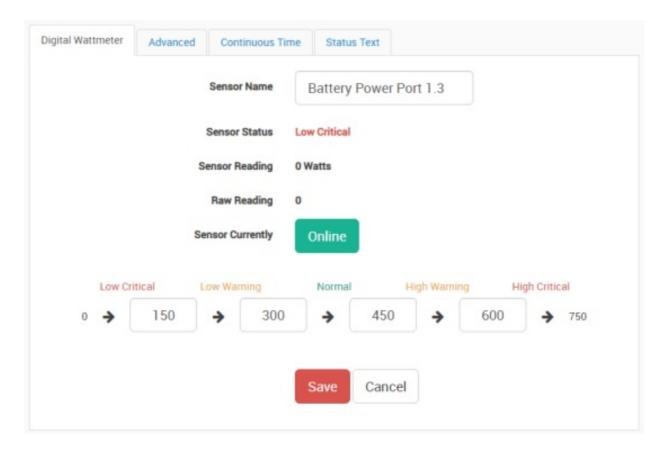
The configuration is similar to a Digital Wattmeter sensor. You can only customize the sensor name and reading thresholds.
