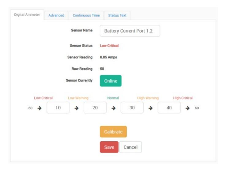
The configuration is similar to a Digital Ammeter sensor.
