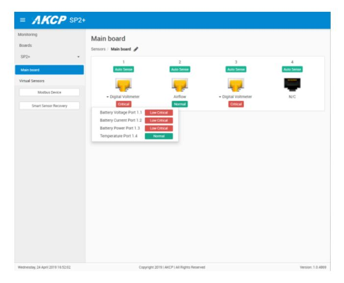
When connected to a sensor port on the base unit, the BMS will appear as a Digital Voltmeter type, with multiple sensors
