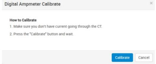
**Note:** the sensor arrives pre-calibrated from the factory, so usually this is not necessary. **Current calibration process:**
