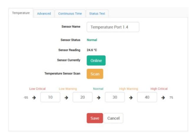
The configuration is exactly the same as with any other Temperature sensor. You can only customize the sensor name and reading thresholds.
