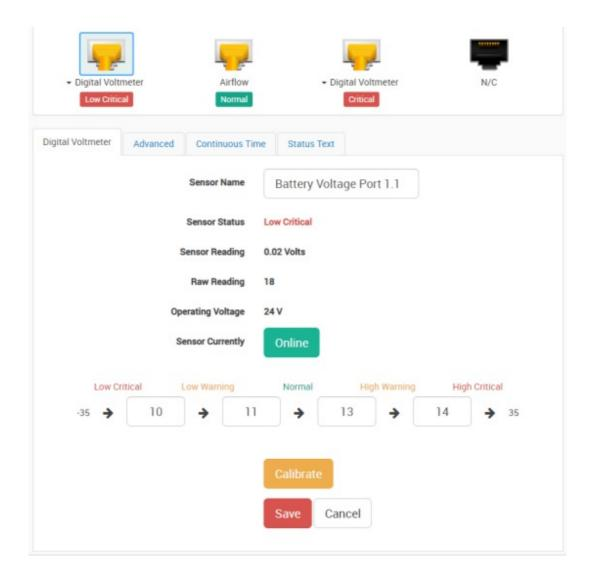
The configuration is similar to a Digital Voltmeter sensor.
