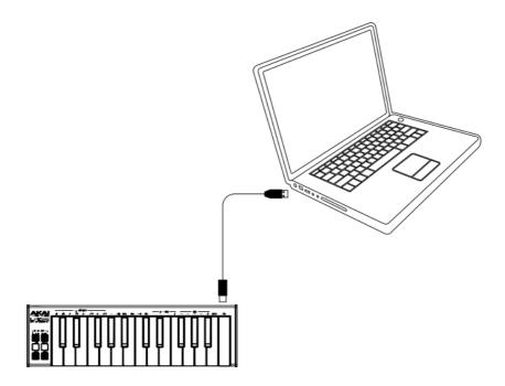
**USB Connectivity & Power:** Use a standard USB cable to connect LPK25 mk2 to your computer.
