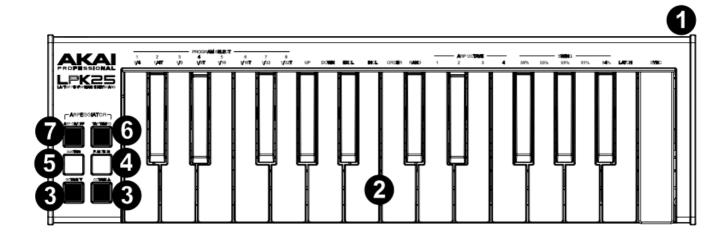
1. USB Port (Rear Panel): Use a standard USB cable to connect this USB port to your computer. The computer's
