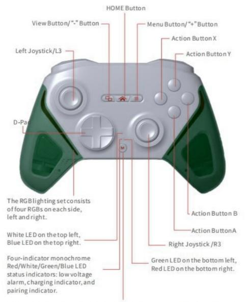
The motor setting button has: rapid fire function and motor vibration adjustment, and in NS, it is the screenshot function.
