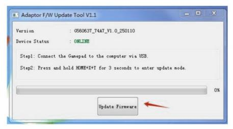
3. During the upgrade process, ensure the data cable remains stably connected. Once the upgrade is complete, the display will show as in the image below:
