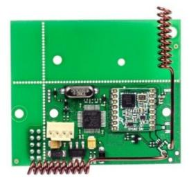
**uartBridge** is the module for integration with third-party wireless security and smart home systems. A wireless network of smart and secure Ajax detectors can be added to a third-party security or smart home system through the UART interface.
