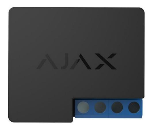
Relay is a wireless, low-voltage relay featuring potential-free (dry) contacts. Use Relay to remotely switch on/off appliances powered by a 7–24 V DC source. Relay can operate both in pulse and bistable mode. The device communicates with a hub via Jeweller radio protocol. In the line of sight, the communication distance is up to 1,000 m.
