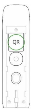
3. Turn on the detector by holding its power button for 3 seconds.
