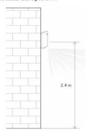
Installing the detector at any other height will narrow the detection zone, affecting the quality of motion detection. Keep in mind that MotionProtect Curtain does not detect movement behind the glass. Therefore, do not install the detector in places where glass structures may block its range of view, e.g., in places where an open window may obstruct the devices.
