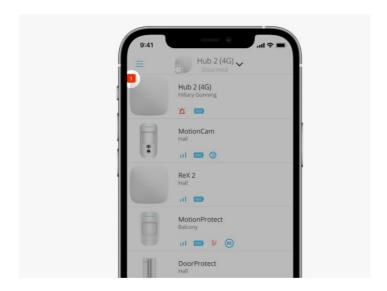
If a hub fault is detected (e.g., no external power supply is available), a faults counter is displayed on the device icon in the Ajax app.
