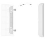
If use screwdrivers, set the speed to the minimum so as not to damage the SmartBracket mounting panel during installation. When using other fasteners, make sure they do not damage or deform the panel. To make it easier for you to mount the detector or magnet, you can pre-drill the screw holes while the mount is still secured with double-sided tape.
