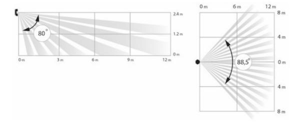
If the detector is not installed at the recommended height, this will reduce the area of the motion detection zone and impair the operation of the function of ignoring animals.
