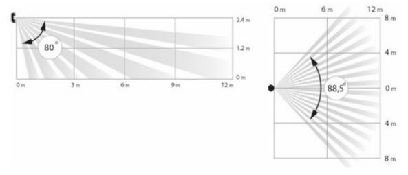
If the detector is not installed at the recommended height, this will reduce the area of the motion detection zone and impair the operation of the function of ignoring animals.3
