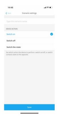
When cony, which is in pulse mode, the **Device Action** setting is not available. During the scenario execution, this relay will close/open the contacts for a set time. The operating mode and pulse duration are set in the. Relay settings
