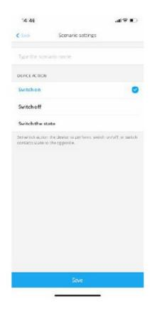
**Note:** When configuring a scenario for Relay, which is in pulse mode, the Device Action setting is not available. During the scenario execution, this relay will close/open the contacts for a set time. The operating mode and pulse duration are set in the Relay settings.
