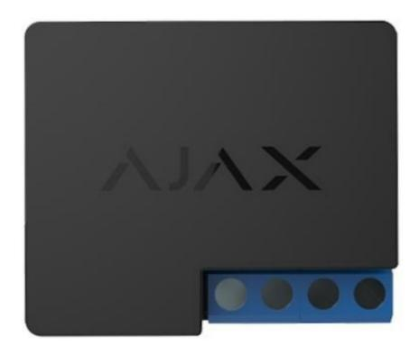
Relay is a wireless, low-voltage relay featuring potential-free (dry) contacts. Use Relay to remotely switch on/off appliances powered by a 7–24 V DC source. Relay can operate both in pulse and bistable mode. The device communicates with a hub via radio protocol. In the line of sight, the communication distance is up to 1,000 m.
