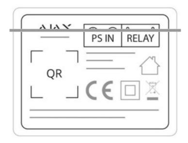
**PS IN terminals**— "+" and "" contact terminals, 7-24 V DC input power supply. **Relay terminals** output potential-free terminals.
