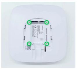
5. Remove the screws attaching the boards to the device body.
