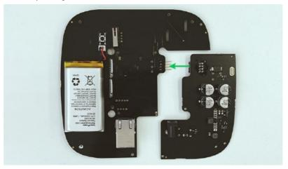
**Please note:** the board contacts should be plugged in the bottom row of the connector(closest to the board). When connected correctly, the boards are on the same level.
