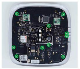
6. Carefully remove both boards, keeping them in the same plane and not disconnecting them. There is a connector between boards: do not break it.
