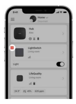
When a device identifies a fault (for example, there is no connection with the hub), the Ajax app displays a fault counter in the device feld.
