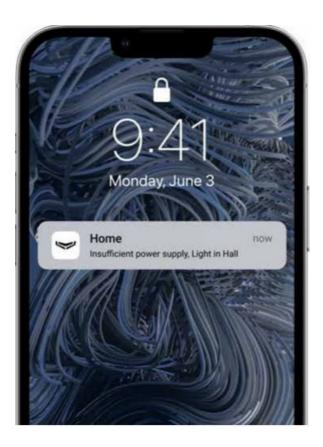
LightSwitch regularly measures the switching current. If LightSwitch controls the power of a lighting device with insu?cient power (up to 5 W), the system will notify the users of the Ajax system. In this case, it is necessary to replace the lighting device with a similar one with higher capacity or to connect a bundled capacitor in parallel with the lighting device.
