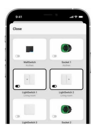
The lighting also can be controlled in the Control menu. To do this, go to the Control menu and swipe up. All control devices added to the hub will appear in the list. Click on the switch in the LightSwitch feld, and the state of the device's contacts will change to the opposite. The lighting will switch on or off.
