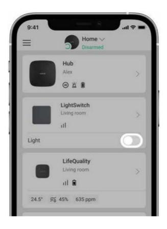
Press the switch in the LightSwitch feld in the Devices menu in the Ajax app, and the state of the switch contacts will change to the opposite; lighting will be switched off or on. This way, system users can remotely control the lighting. For example, switch on the light in the room in advance before entering the room.
