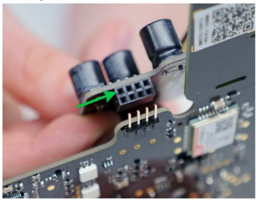
10. Reassemble the boards and the device body then tighten the screws.
