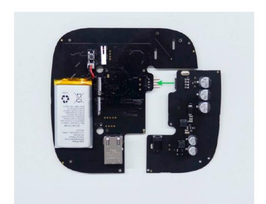
9. Connect 12V PSU for Hub 2 to the mainboard using the eight-pin connector between them. Do not warp or bend the antennas while replacing the board: this can cause the device to malfunction.
