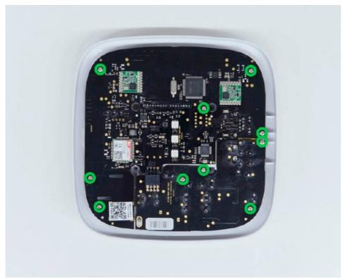
6. Remove the screws attaching the boards to the device body.
