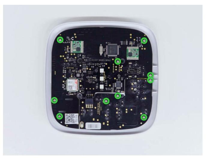
6. Carefully remove both boards, keeping them in the same plane and not disconnecting them. There is a connector between boards: do not break it.
