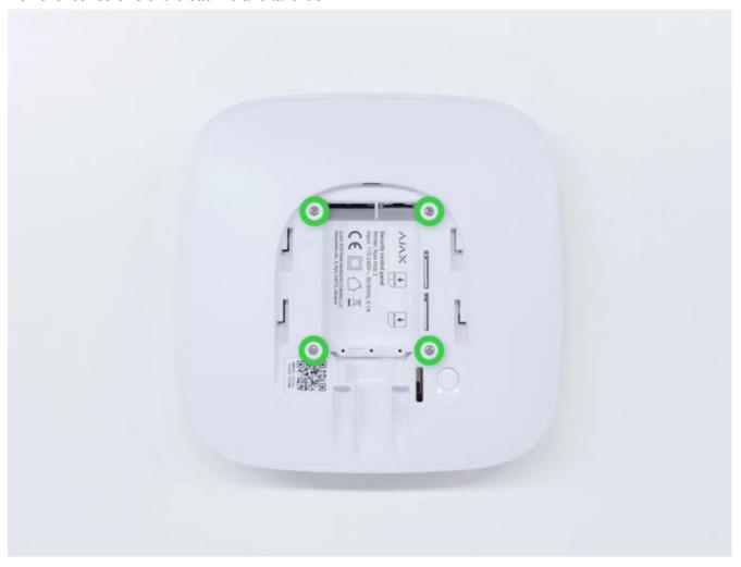
5. Remove the screws attaching the boards to the device body.
