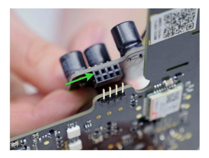
9. Reassemble the boards and the device body than tighten the screws.
