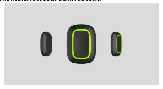
The button is a wireless panic button with protection against accidental press and additional mode to control
