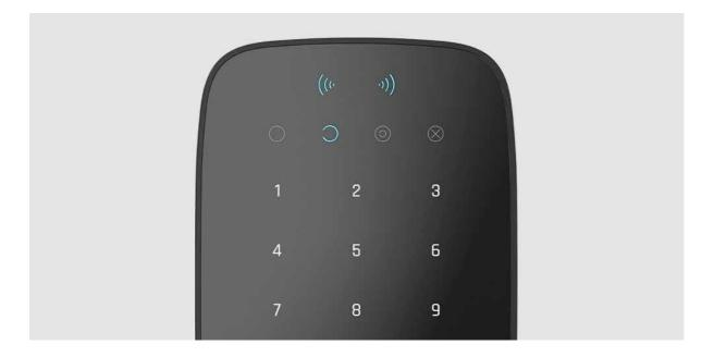
You can use the KeyPad Plus without ambient lighting as the keypad has a backlight. The pressing of the buttons is accompanied by a sound signal. The backlight brightness and keypad volume are adjustable in the settings. If you do not touch the keypad for 4 seconds, KeyPad Plus reduces the backlight brightness, and 8 seconds later
