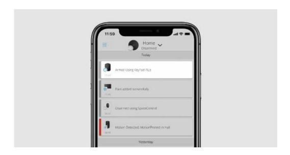
KeyPad Plus is locked for the time specified in the settings if an incorrect password is entered three times in a row within 1 minute. The corresponding notifications are sent to users and to the monitoring station of the security company. A user or PRO with administrator rights can unlock the keypad in the Ajax app.
