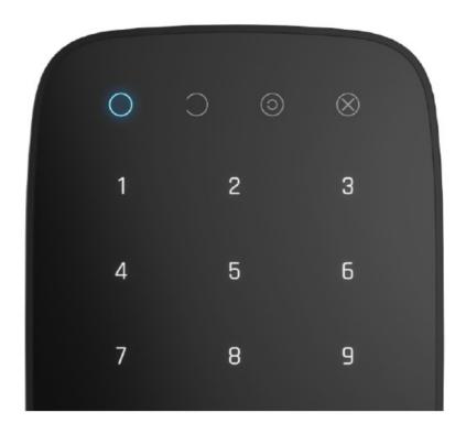
When touching KeyPad, it wakes up highlighting the keyboard and indicating the security mode: Armed, Disarmed, or Night Mode. The security mode is always actual, regardless of the control device that was used to change it (the key fob or app).
