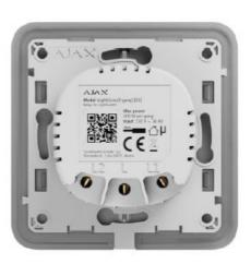
A single LightSwitch consists of two elements: a LightCore relay and a SoloButton touch-sensitive panel.
